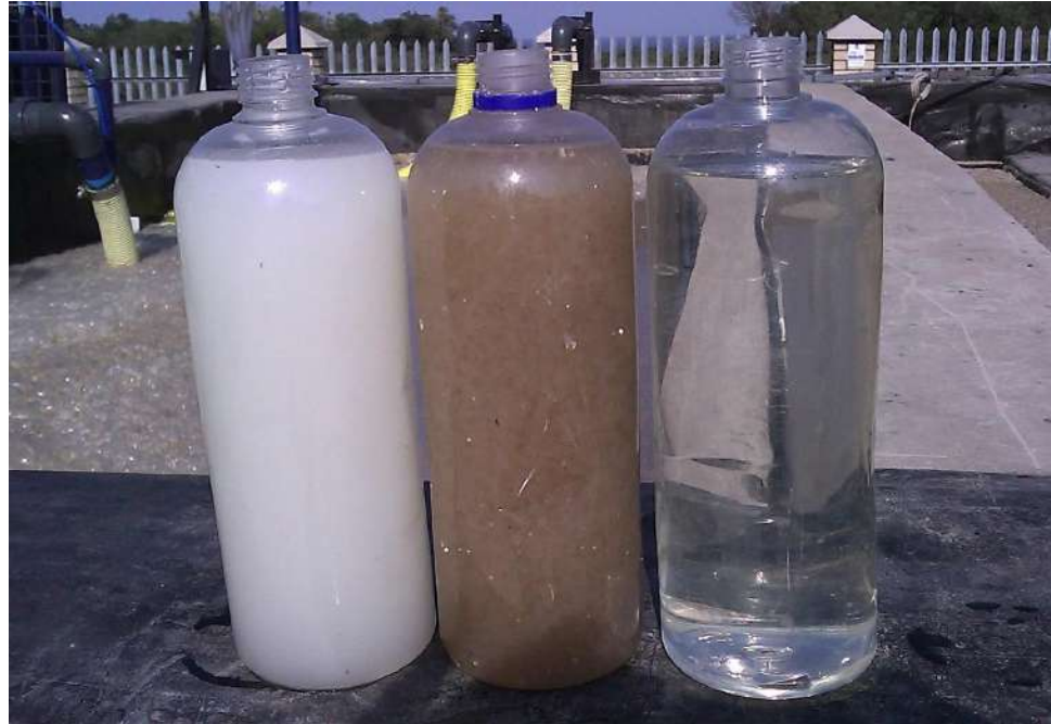
Raw waste water | MBR Reactor Water | Treated Waste Water (with Bacteria)
