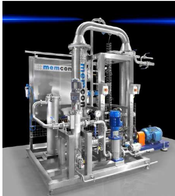
Typical ceramic UF membrane plant for treating 50 t/day spent caustic
